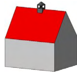
LoD3: detailed building installation
